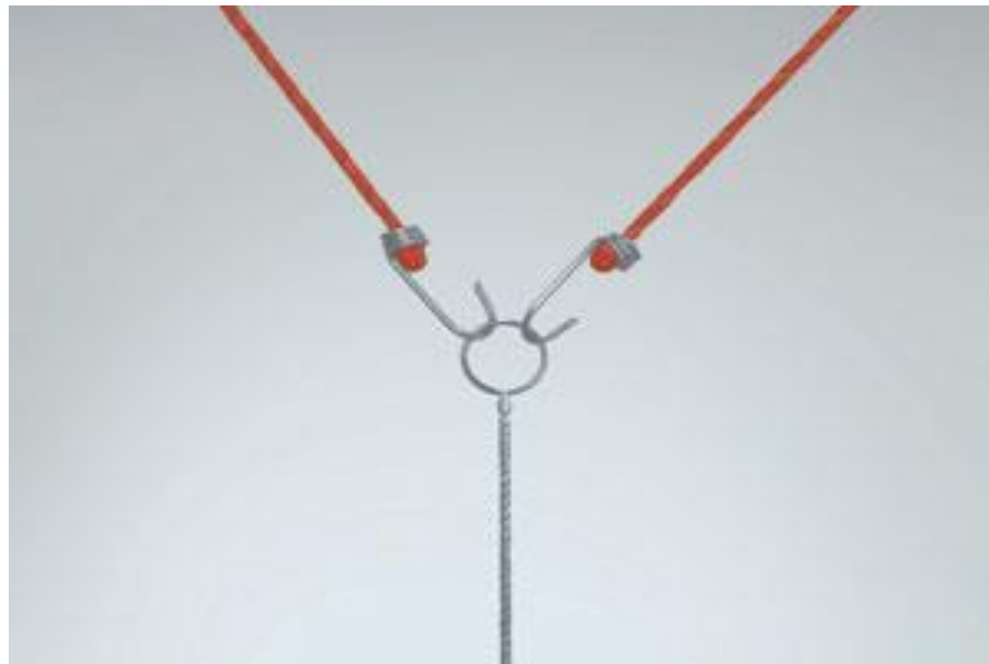
Fig.1, Three forces act on the ring. Since these forces all meet at point, then for any force analysis, we can assume the ring to be represented as a particle.
