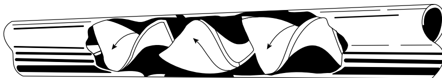
Figure 10.53. Static mixer (Kenics Corporation)
