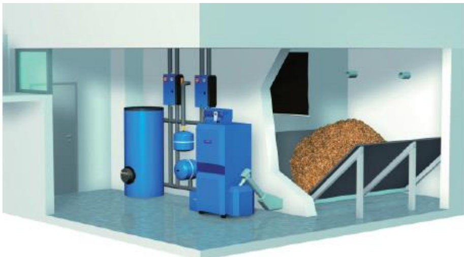
Figure 12.9 Wood pellet heating with pellet store. Source: BBT Thermotechnik GmbH.
